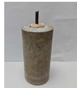
ข) Fly ash-waste glass powder alkali-activated mortar
